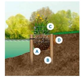
Fig 1. Shows a cross section of installation of the coir.
