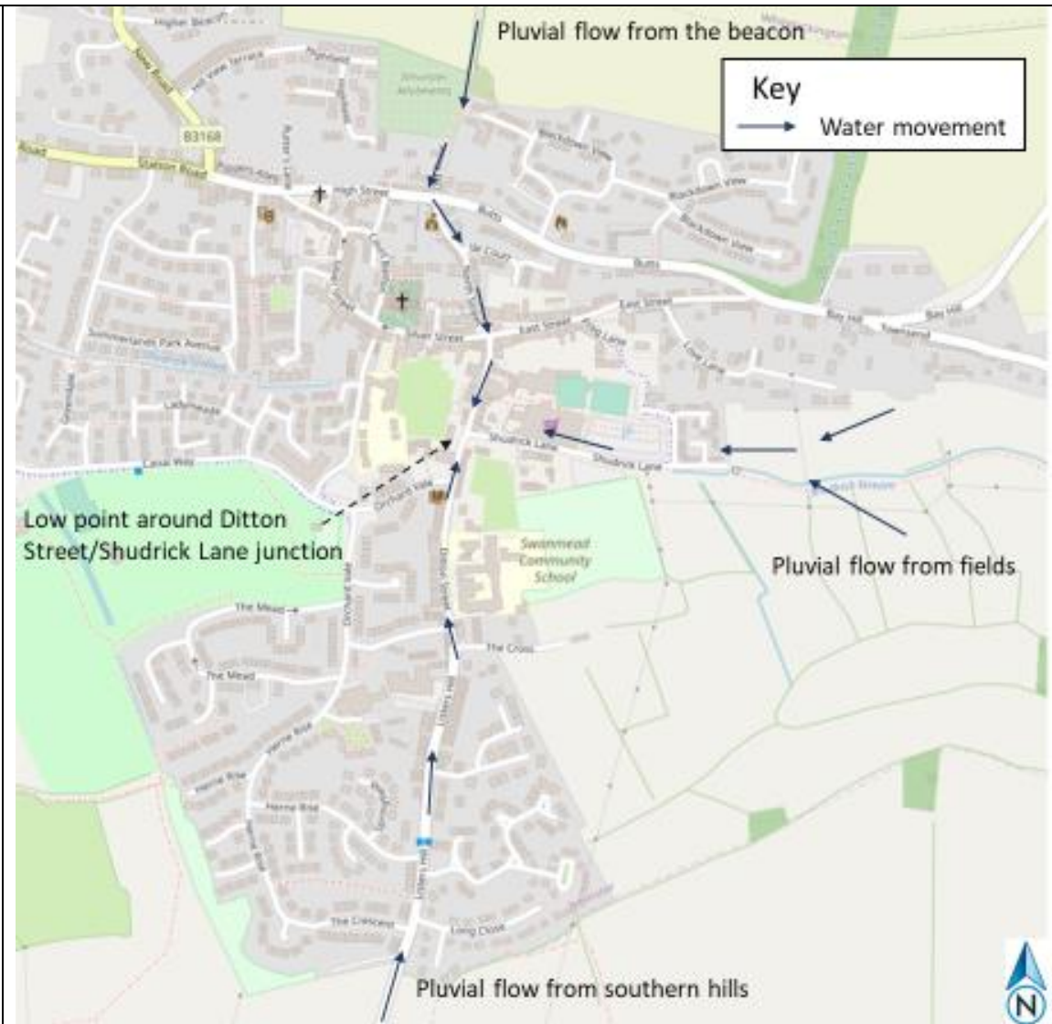
Figure 31: Pluvial flows around east Ilminster
